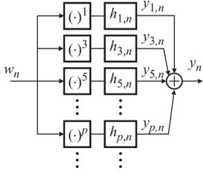
Fig. 1. Discrete baseband model of the PWM modulator.
