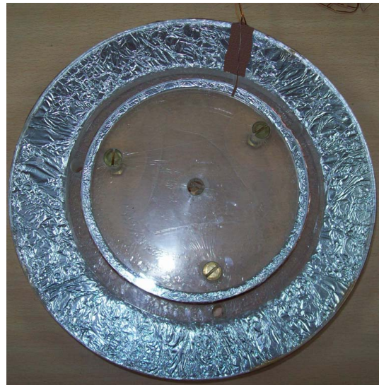
Figure. 5. Shielded MF_{AC} and MF_{DC} coils that compose the Helmholtz pairs.
