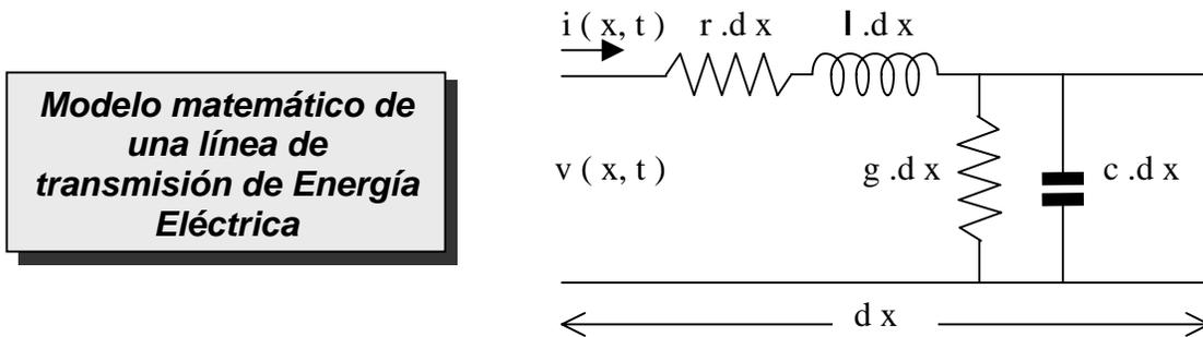
$$\left\{ \begin{array}{l} \frac{\partial v(x, t)}{\partial x} = r \cdot i(x, t) + l \frac{\partial i(x, t)}{\partial t} \\ \frac{\partial i(x, t)}{\partial x} = g \cdot v(x, t) + c \frac{\partial v(x, t)}{\partial t} \end{array} \right.$$
