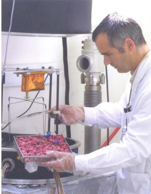
Figure N° 8: Lyophilization stands for drying in a cold atmosphere. Lyophilization is often used to preserve biological materials. It is especially used to preserve food.
