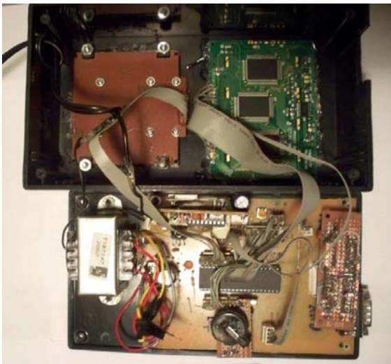
Fig A-3 Despiece modulo control
