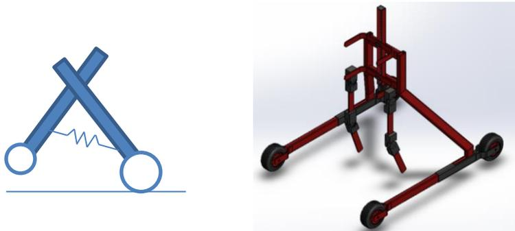
**Figure 4 – (a) Schematic wheels and spring (b) Added passive exoskeleton**
